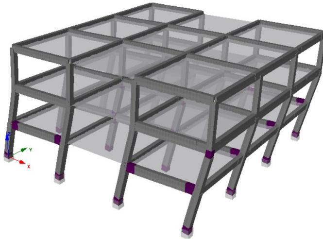
Fig. 4- Load step for the collapse, controlled by the ultimate rotations at the end of first-floor beams and columns (ductile failure)
